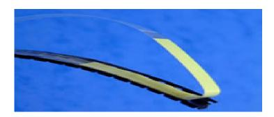
Cover tape extenders are used when a reel of SMT components doesn't have a leader at the beginning of the reel.
